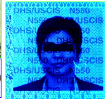
Magnification of the printed photo area when viewed with UV light. The UV security fibers and security text “DHS/USCIS N550” and “N550 DHS/USCIS” are visible in the photo block area. (Note: these features are obscured in the attached photo version).
