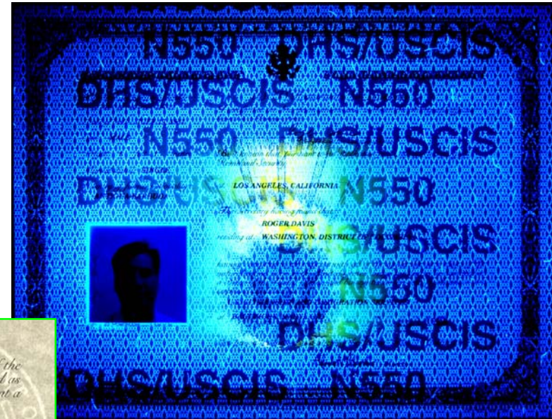
Magnification of the printed photo area when viewed with UV light. The UV security fibers and security text “DHS/USCIS N550” and “N550 DHS/USCIS” are visible in the photo block area. (Note: these features are obscured in the attached photo version).
