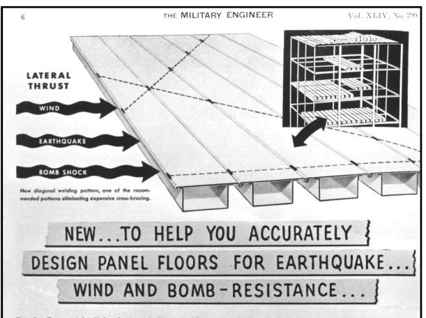
By using Fenestra's\* cellular sheet steel "D" and "AD" Building Panels or Holorib Root Deck, following the methods given in Fenestra's "Seismic Building Design" brochure, you can stiffen your buildings against earthquake, wind and bomb shock. You can thus take full advantage of another asset of light-gauge steel construction and save building time, labor, materials and money.
